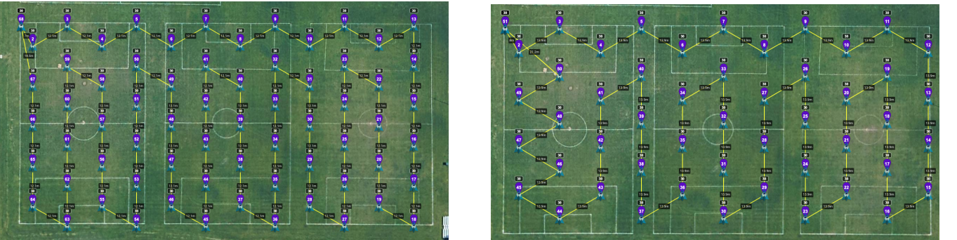
Figure 1: Two circumstances of GPS way-points for drone covering a rectangular field using hexagonal tessellation
